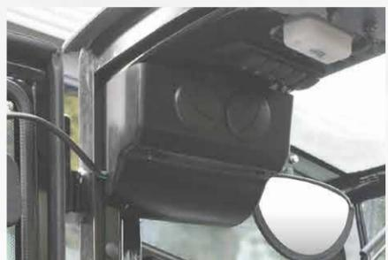
Equipped with a fully enclosed cab, it has excellent performance in rust prevention, short circuit prevention, waterproofing, and insulation, meeting the usage environment of  $-30^{\circ}\text{C}$  (test data: operating in a  $-30^{\circ}\text{C}$  cold storage, the cab temperature is higher than  $0^{\circ}\text{C}$  )
