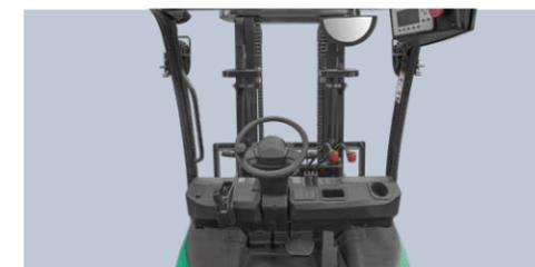
The wide-view mast with optimized design is unlikely to obstruct the operator's line of sight. The enlarged opening size of the fork carriage enables a wider view.
