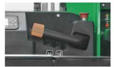
The acceleration joystick is equipped with a sensing switch for the standard configuration to prevent mis-touch during operations.
