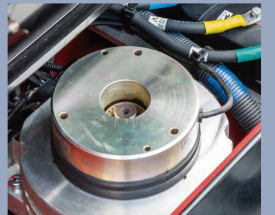
Electrical Park Brake (EPB) system
